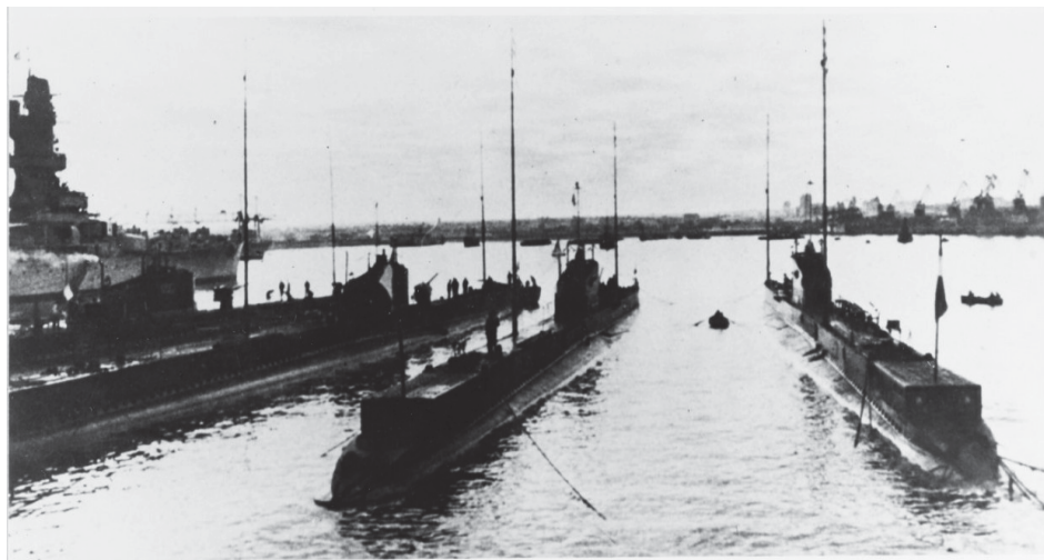
Figure 3. Four 1500-tonne type fleet submarines at Toulon or Marseilles in the 1930s, with the heavy cruiser Algérie on the left. Note the trainable box mounts for the four stern torpedo tubes. A similar triple mount was located abaft the conning tower as well. Courtesy of www.history.navy.mil .
